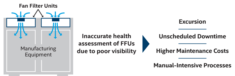
Figure 1. Manufacturing equipment often includes fan filter units (FFUs), which draw in fab air and push it through high-efficiency particle filters. This keeps the air inside the machine cleaner by filtering it and reducing particles in the machine's clean chambers. Detecting FFU health is often a manual process, which makes predicting failure difficult.
